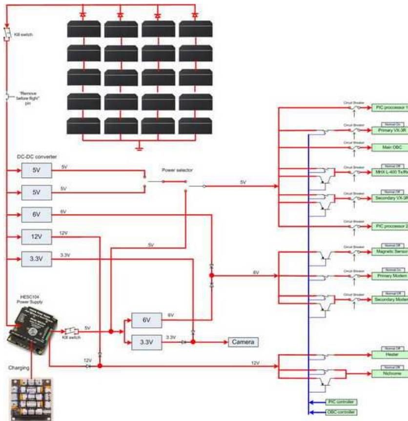
Figure 11. Power Supply Unit design with redundant power sources and circuit-breakers to protect major components from latch-up
