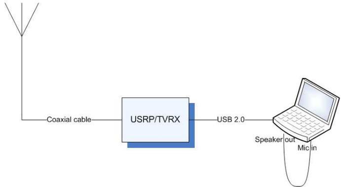
Figure 3. Simple ground receiving station setup
