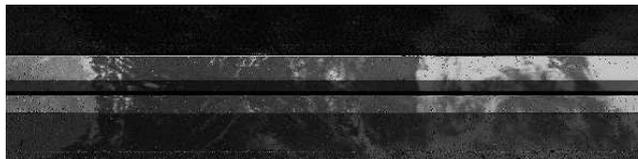
*Figure 5. First signal from NOAA 17 satellite, Feb 04, 2009, different bands of shades are due to unequal volume adjustment during the recording*
