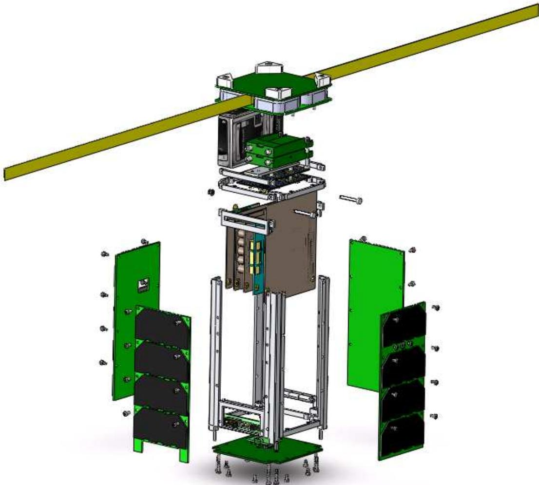
Figure 10. Exploded view of F-1 nanosatellite
